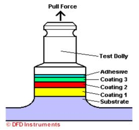
Adhesion testing to ASTM D4541 is very much like conventional tensile testing, the only difference is that the test sample for ASTM D4541 is very short.
